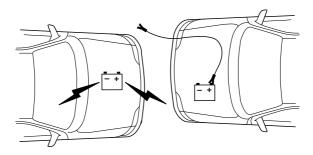
1. Connect the positive (+) jumper cable to the positive (+) terminal of the discharged battery.
